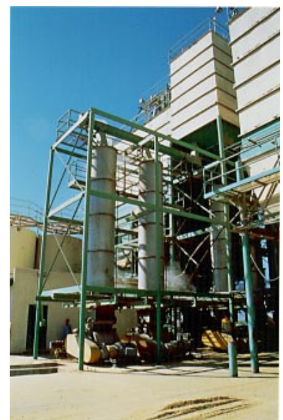
Fig. 8. Steam cabinet towers in Arizona used for steam-flake milling to decontaminate wheat infected and/or infested with Karnal bunt teliospores.
