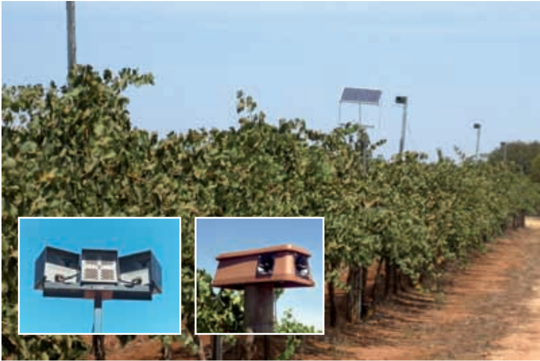
Figure 4.8: Electronic speakers used to broadcast sounds to scare birds away from crops. Photo: R. Sinclair. Inset photos left: T. Bentz, right: R. Sinclair.
