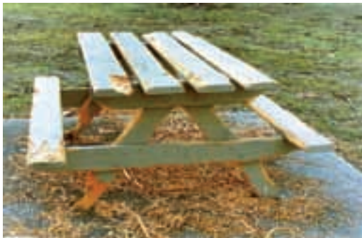
Figure 2.3: Sulphur-crested cockatoo damage to oregon picnic table, Bundoora Park, Victoria. Photo: I. Temby.
